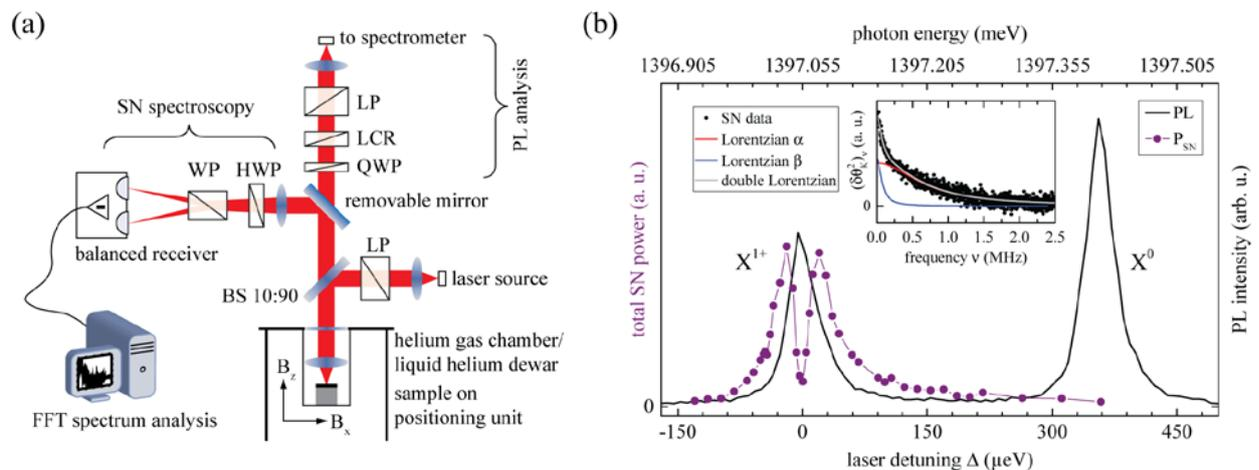
Fig. 1: (a) Experimental setup for PL analysis and SN spectroscopy on a single QD. (b) PL spectrum of a single QD showing the optical transition of the neutral exciton ( $X^0$ ) and the positively charged trion ( $X^{1+}$ ). The purple data points depict the SN power measured as a function of probe laser detuning with respect to the trion resonance. The inset shows a typical SN frequency spectrum revealing two Lorentzian noise contributions.
