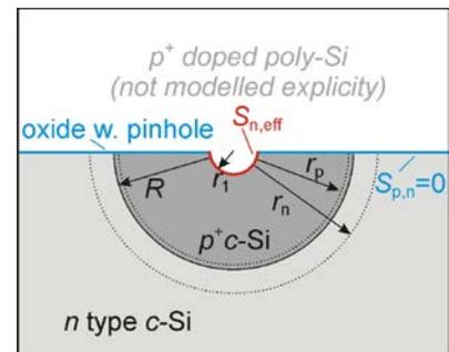
**Figure 1:** Illustration of an analytical model [3] describing the current flow in poly-Si/c-Si junction
