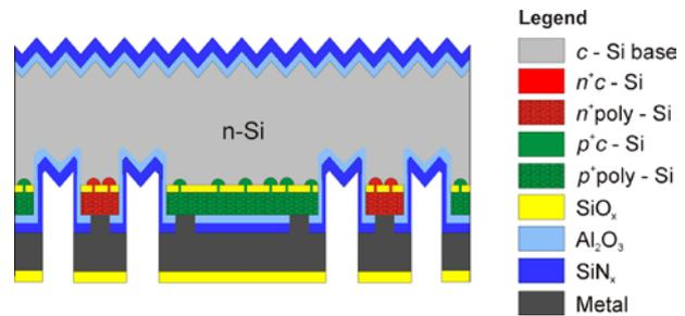
**Figure 3:** Back-junction back contacted Si solar cell structure with carrier selective poly-Si/c-Si junctions.
