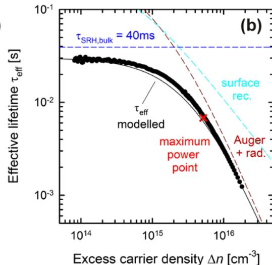
**Figure 2:** (a) Fabrication process of poly-Si/c-Si junctions, (b) Effective lifetime vs. excess carrier density, measured by the photo conductance decay method. The cyan line represents the limitation induced by recombination at the poly-Si/c-Si junctions.
