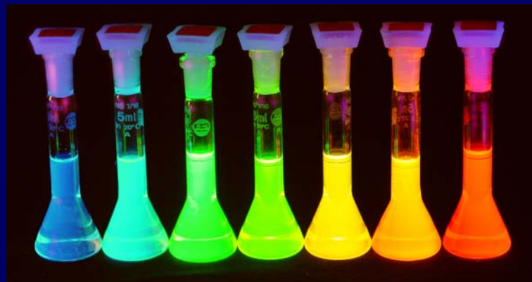
PL of CdSe/ZnS core-shell nanocrystals in chloroform.
