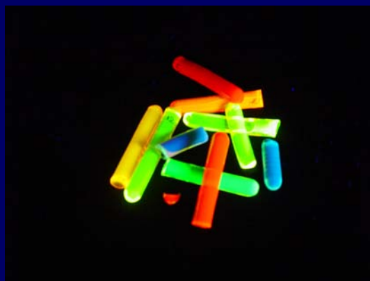
Composites of CdSe/ZnS and CdSe/CdS nanocrystals and poly(laurylmethacrylate) (PLMA)
