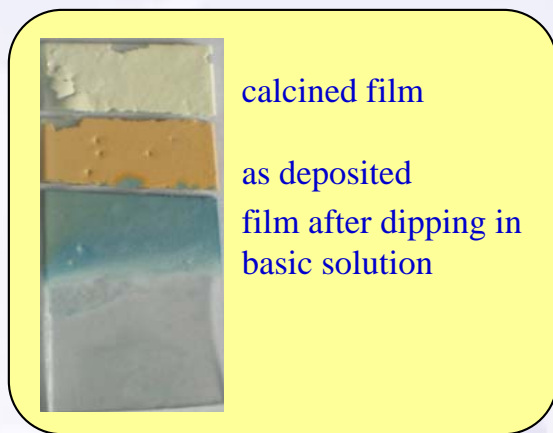
film deposited with BTB at 80 °C
