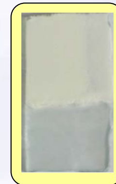
film deposited with SDS at 80 °C
