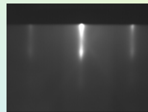
(1x1)-Si(111) (after 4 ML Si deposition)
