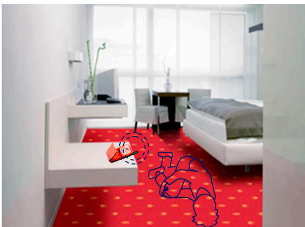
Figure 4: An alarm will be triggered, if a person falls down on the floor and remains motionless.
