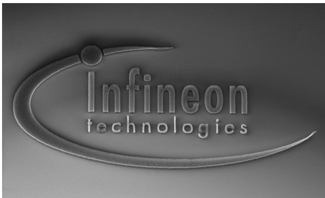
Figure 10: Infineon logo composed of millions of vertically grown entangled nanotubes on top of a catalyst layer (not visible) that was patterned by lithography.
