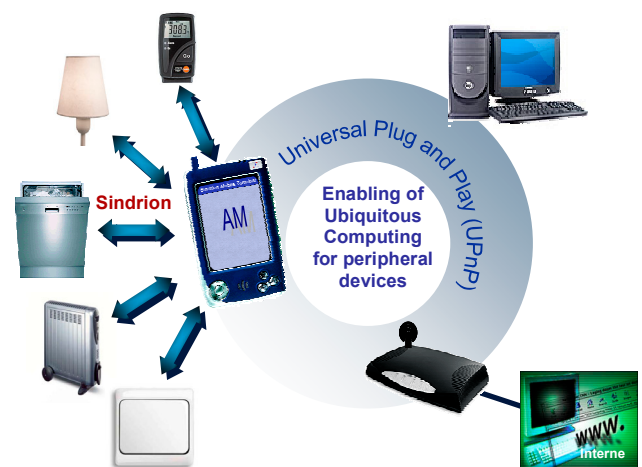
Figure 8: Sindrion Transceivers as part of a UPnP Distributed System.
